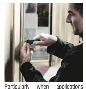
applications involve sensitive materials or high quality surfaces are involved, bits with a diamond coating ensure that work is done safer, faster and at lower cost.
