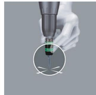
The free-turning sleeve allows screw steadying at the start of the screwdriving process. This makes it easier to apply the tool to the screw and prevents slipping. It can also be used as a short extension for 1/4" applications e.g. in combination with the Wera Zyklus Ratchets.
